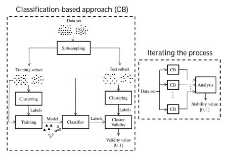
Figure 6.15: Classification-based approach (left), and iterating the process for several train and test sets (right).
